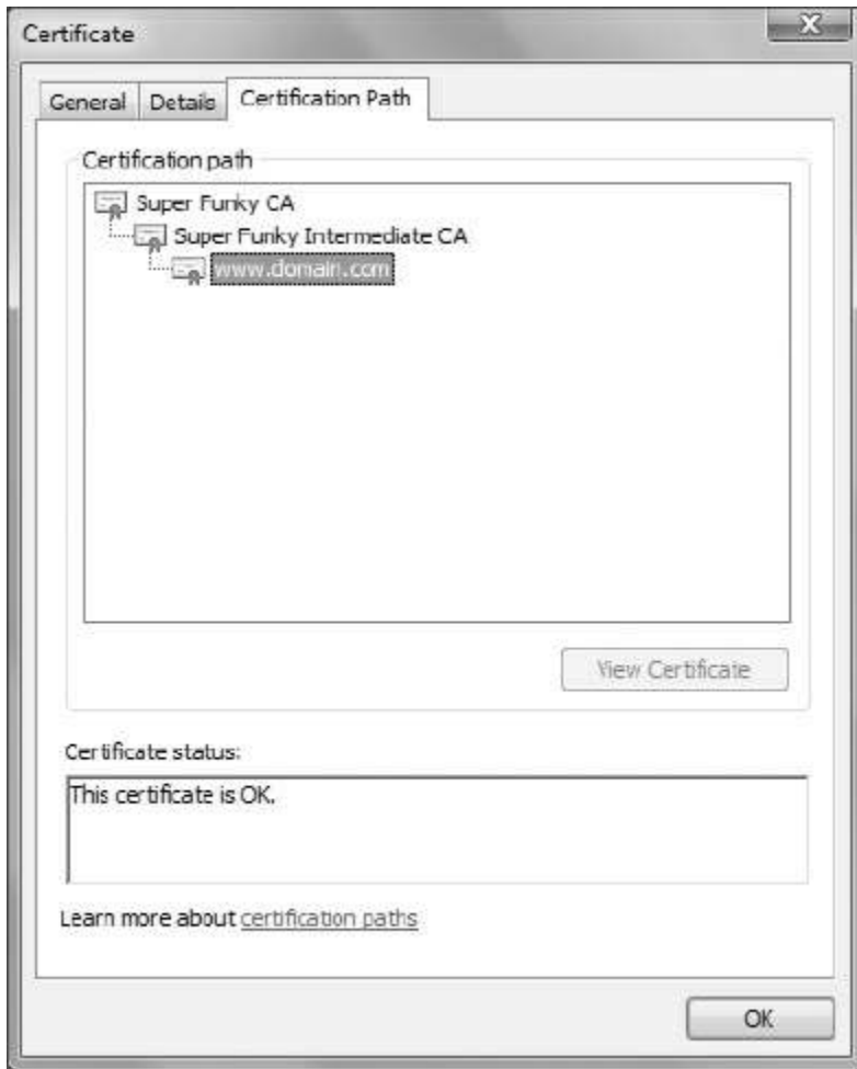
Figure 7-21: The chain of trust for www.domain.com
